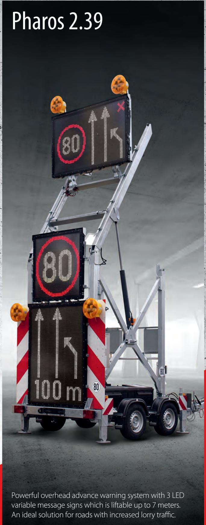
Powerful overhead advance warning system with 3 LED variable message signs which is liftable up to 7 meters. An ideal solution for roads with increased lorry traffic.
